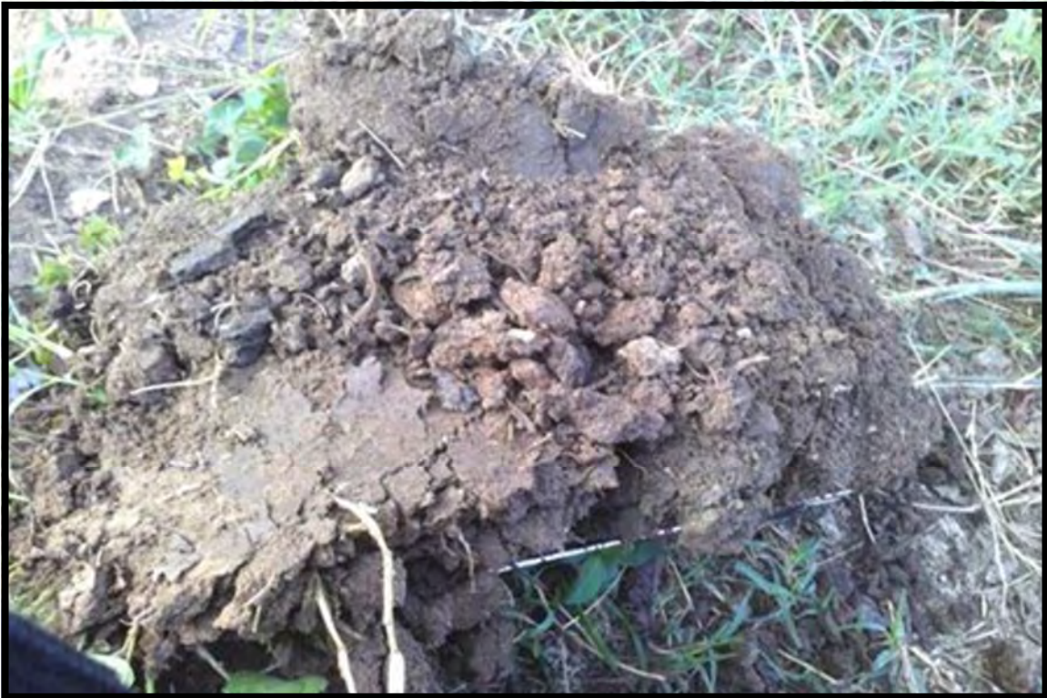
Photo 6 : View of WTP-2 within WTL2. Soils were hydric with a matrix of 10YR4/2 and redox concentrations of 10YR 4/6.
