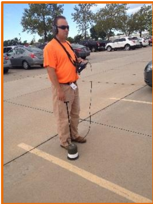
Figure 8. Pinpointing Phase – Our crew will utilize computer correlators and electronic ground microphones to pinpoint leaks that are localized. When correlators are used, the results will be verified using the ground microphone.
